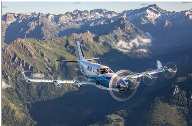
Daher's TBM demonstrator is large enough to integrate an 800-volt electrical system, turbogenerator and six motors.
