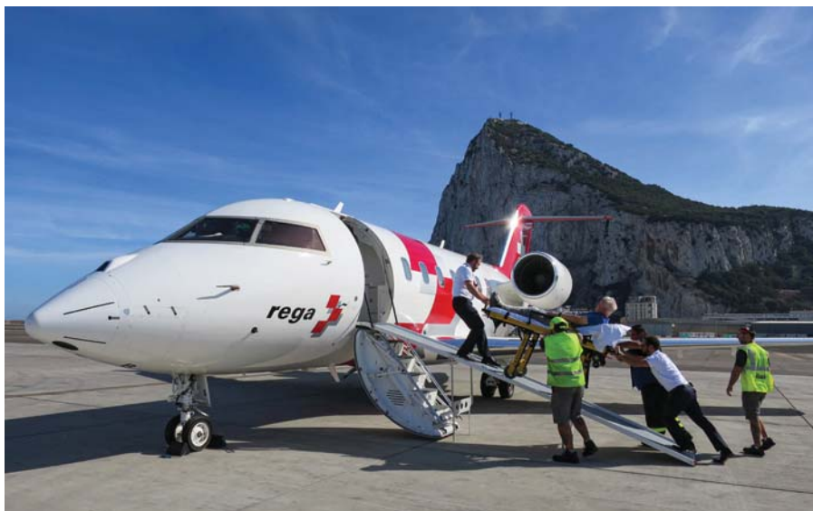
In order to be able to gently load patients lying on a stretcher trolley into and out of their CL-650, Rega has constructed a three-piece ramp which is permanently installed in the jets. The ramp folds into the entrance door of the airplane.
